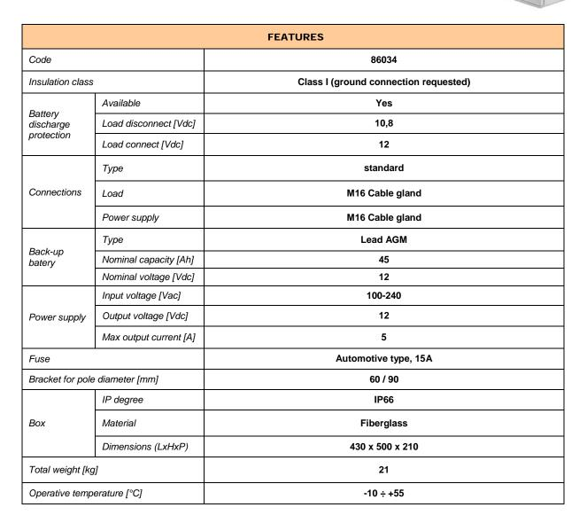
Caution: even though the device is provided with protection against deep discharge of the battery, in case of prolonged absence of mains voltage (over a week) damaging could occur due to self-discharge of the battery.
